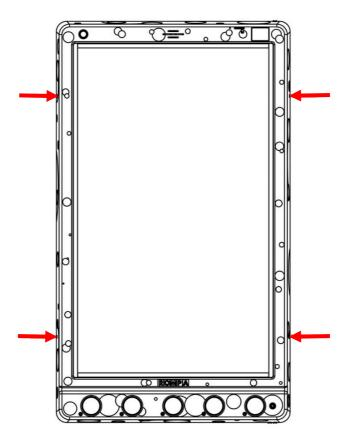
4. Secure both brackets to the wall\* ensuring the centre of the bracket mounting holes line up with the marks just made to ensure the bracket is level when mounting it to the wall. The top bracket mounting holes should line up with the top 2x marks and the bottom bracket mounting holes should line up with the bottom 2x marks.
