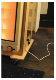
8. Switch on individual products using the switches on one of the long sides, towards the top. The switches have illustrations to indicate which switch corresponds to which product e.g. two switches, one for each of the Deluxe Wall Panels.
